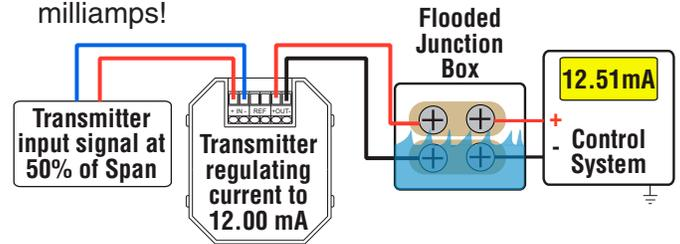
\* The value of the current leak increases when the water in the junction box is contaminated with rust, salt or process chemicals.
