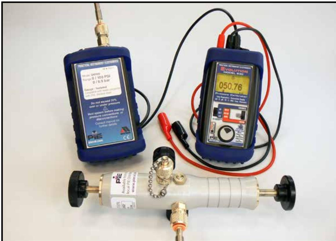
**PIE 830 with Pressure Module, Pressure/Vacuum Pump & Hose**
