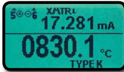
Use the 830 as an *Emergency Transmitter Replacement* to keep the loop running while you grab a replacement from stock and configure it.
