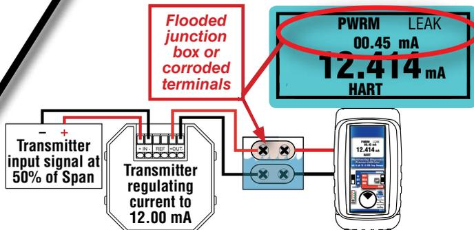
Using the PIE 830 to power up the loop the technician detects a leakage of 0.45 mA - approximately the offset seen in the control room. He walks the loop and opens a junction box releasing a stream of water. The loop is again in control.
