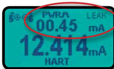
830 detects uncontrolled current in the loop due to a flooded junction box.
