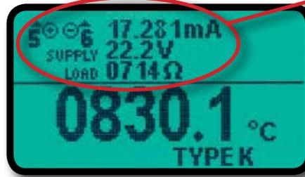
With *LoopScope* running the 830 simultaneously displays the sensor input along with the loop current, power supply voltage and loop load in ohms.
