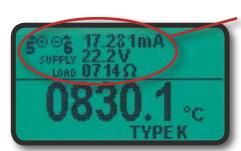
With LoopScope running the 830 simultaneously displays the sensor input along with the loop current, power supply voltage and loop load in ohms.
