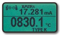
Use the 830 as an Emergency Transmitter Replacement to keep the loop running while you grab a replacement from stock and configure it.
