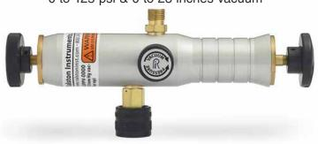
Pneumatic Scissor Hand Pump 0 to 300 psi
