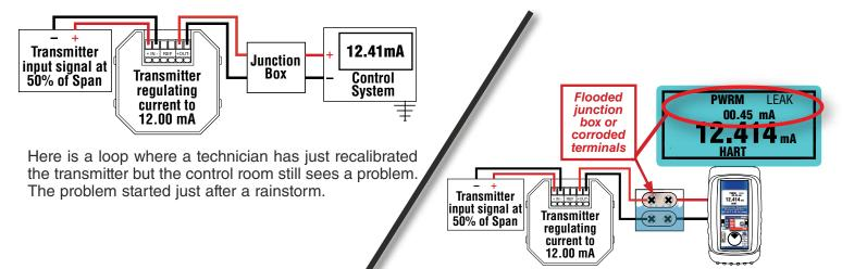
a leakage of 0.45 mÅ - approximately the offset seen in the control room. He walks the loop and opens a junction box releasing a stream of water. The loop is again in control.
