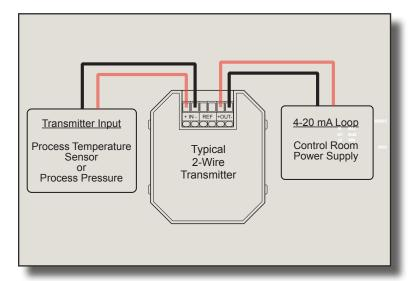
Typical loop with 2-Wire Transmitter
